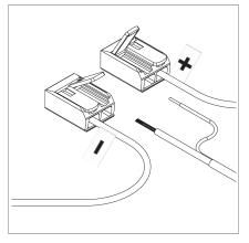
Step 8. Reconnect wire to driver, metal mesh shielding connects to LED- (Black Wire), inner conductor to LED+ (Red Wire). Close terminal blocks to secure connection.
