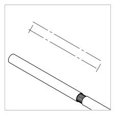
Step 4. Remove outer insulation tube to expose meshed metal shielding. MAKRE SURE TO KEEP THIS INSULATION TUBE
