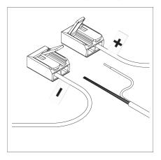
Step 1. MAKE SURE POWER IS OFF. Open terminal blocks to disconnect wires from driver
