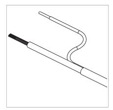
Step 7. Place 1" outer insulation tube over metal mesh shielding. Use a heat-gun or lighter, evenly heat tubing for 10 secs. This will cause tubing to shrink secure tubing over mesh shielding, to act as electrical insulation.
