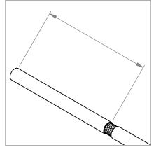
Step 3. Approximately 1" from tip of wire, carefully cut outer insulation to expose meshed metal shielding inside.
