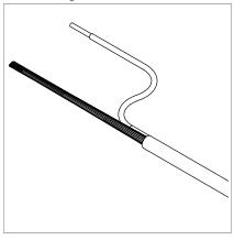
Step 6. Expose inner conductor by removing inner insulation. Reorganize metal mesh shielding.
