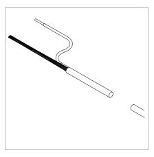
Step 2.Cut off excess wire length
