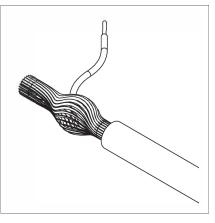
Step 5. Careful push to seperate metal mesh shielding to expose inner wire, take inner wire out from side of metal mesh shielding.
